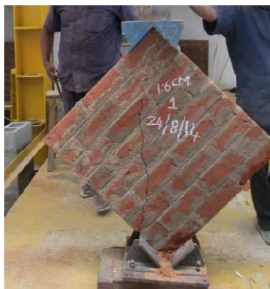
Figure 10: Failure of Diagonal Specimen
