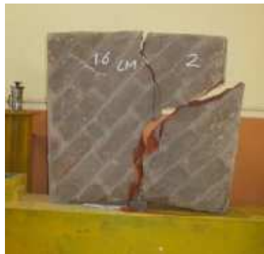
Figure 9: Failure of Specimen with Inclined Bed Joints
